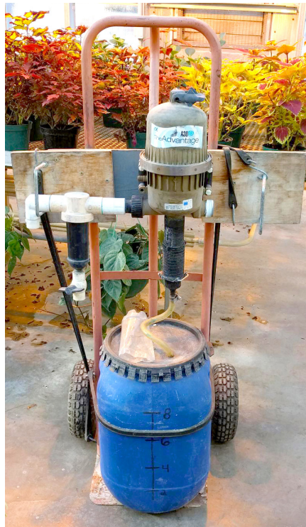
FIGURE 29. Water-powered fertilizer injector.
