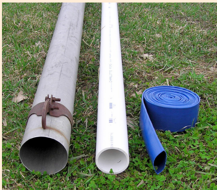
FIGURE 3. From left, aluminum, PVC, and lay-flat pipe materials.
