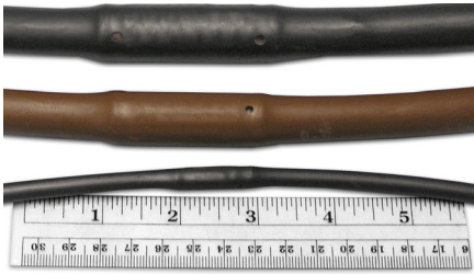
FIGURE 12. Heavy-walled drip tubing for surface or sub-surface applications.
